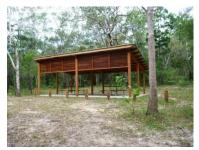
2010. The facilities are in good condition but constructed of timber which will be susceptible to damage. No rubbish bins are in place and rubbish already exists at the site. No signage is evident either relating to the OTL or seeking cooperation on rubbish removal etc.
