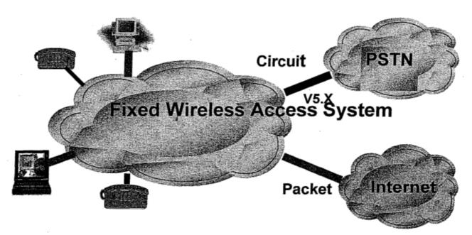
The Immediate Split of Packet and Circuit
