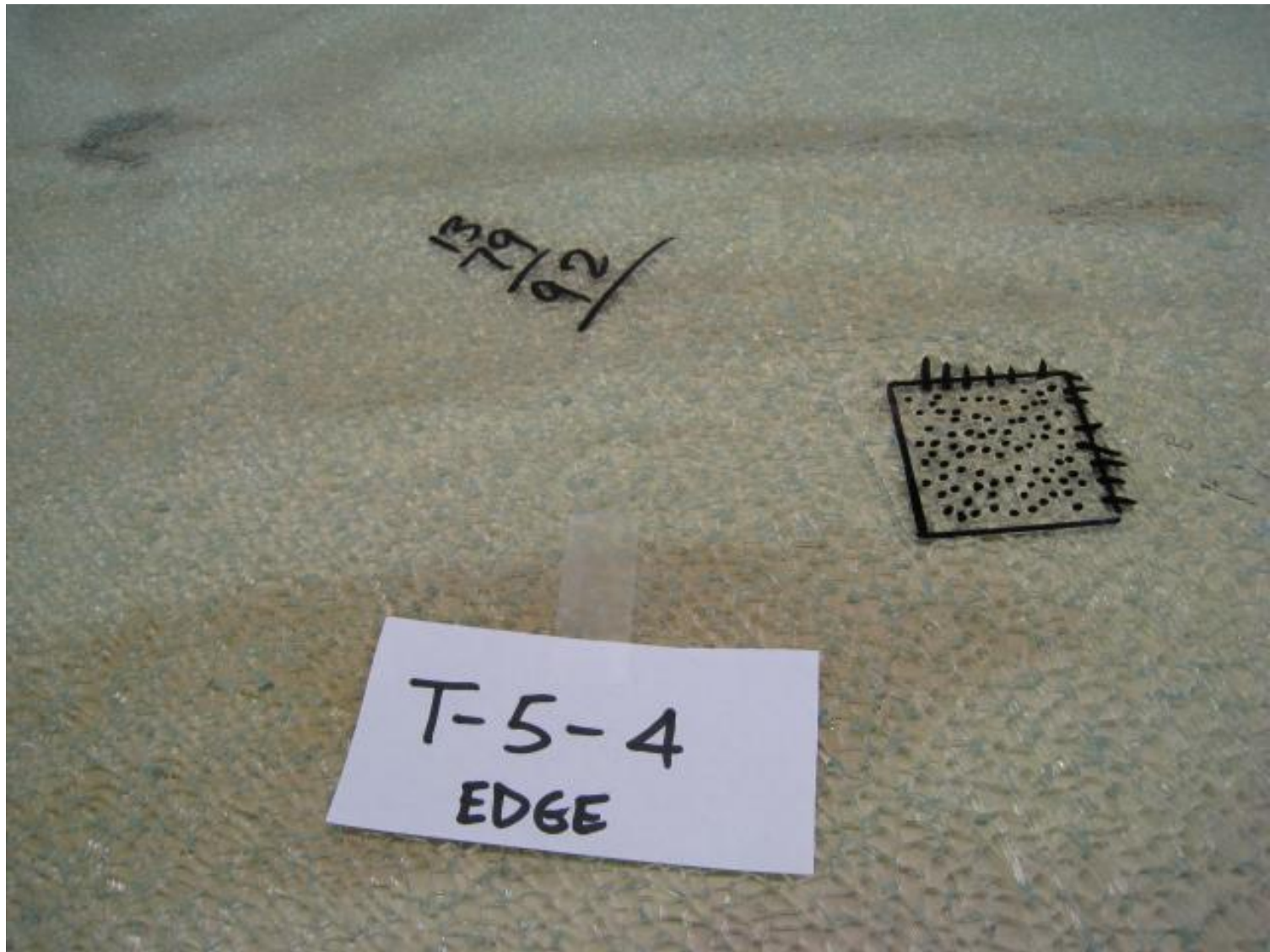
5 mm Sample No.1-4-4; SC 107: Edge Fragmentation - PC 92
