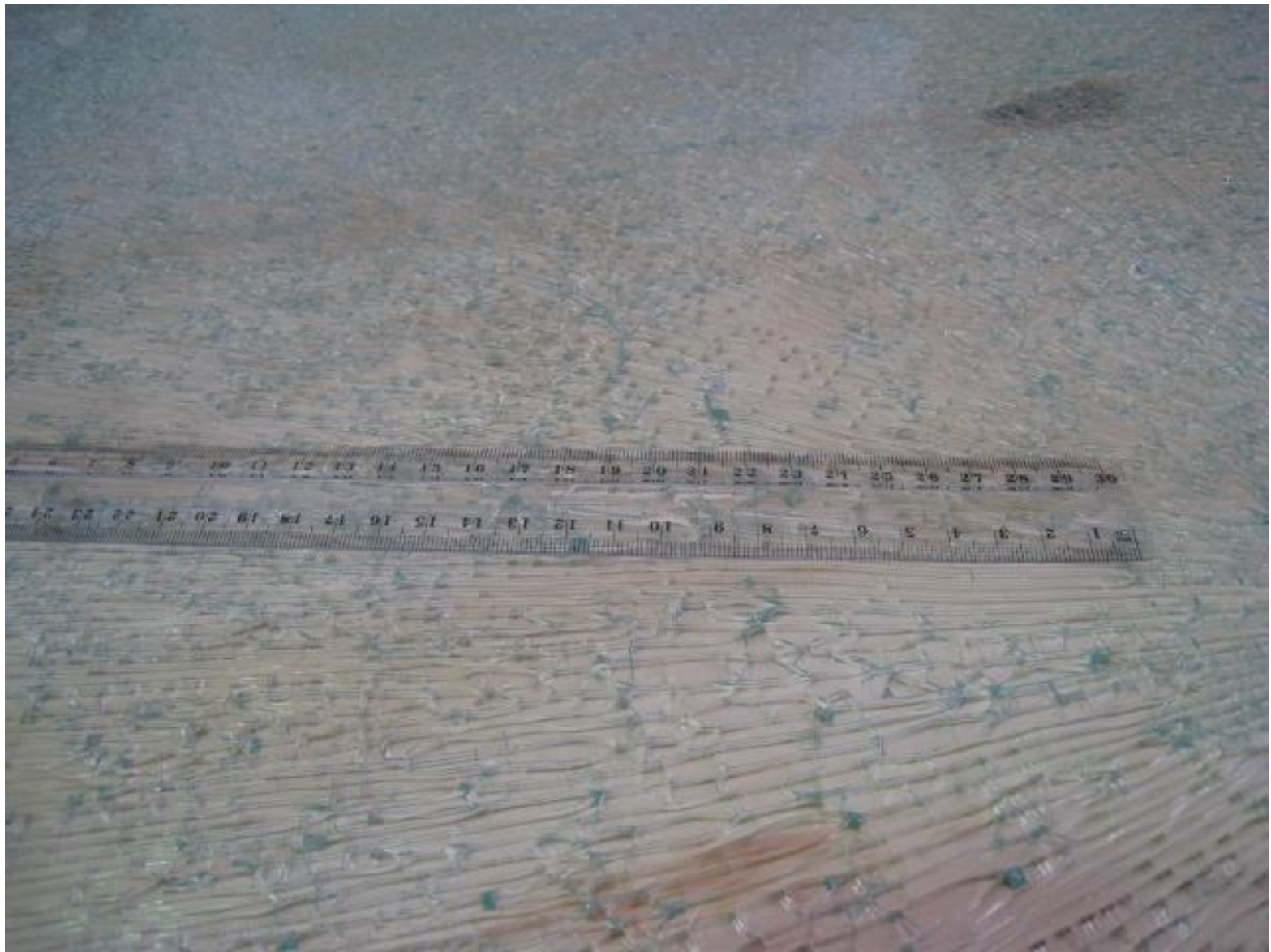
5 mm Sample No. 1_5-1; SC 115: Centre Fragmentation - Longest Particle 135 mm
