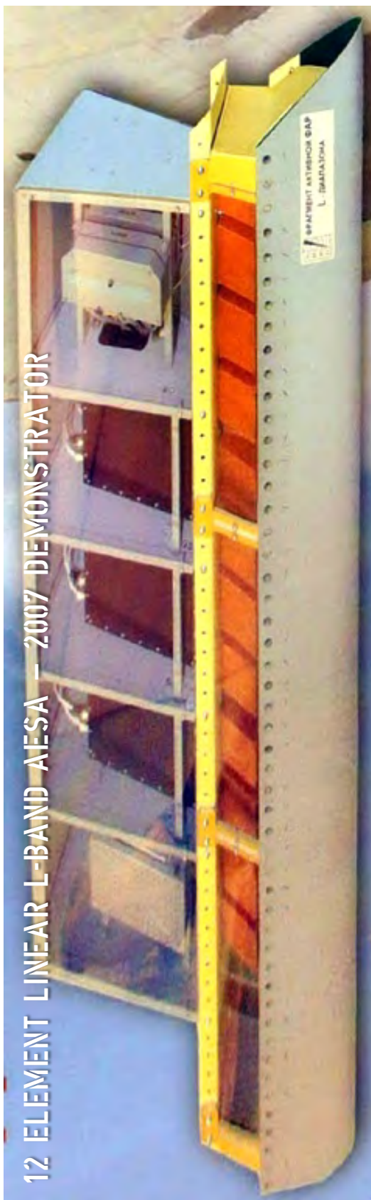
LEADING EDGE AESA INSTALLATION (FLANKER)
