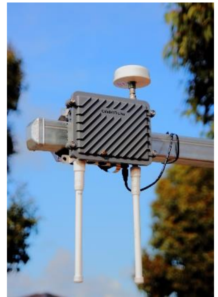
Figure 2: Roadside infrastructure for vehicle-to-infrastructure communications
