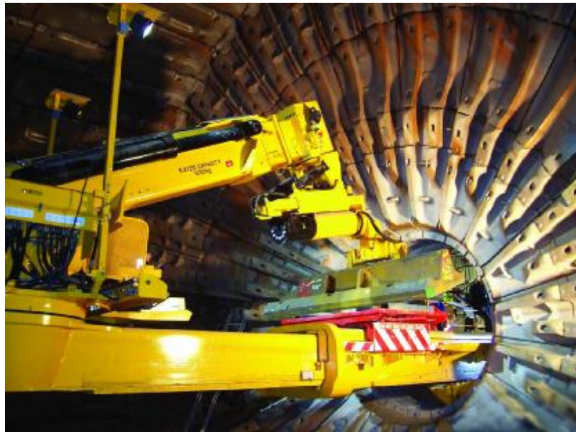
A typical RME Mill Relining Machine
