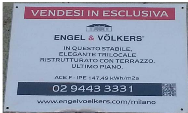
Fig.1: The annual energy consumption of this building is 147.49 kWh/m 2 . Note that the 2012 European Energy Directive mandates 40 kWh/m 2 and year 10 , and 15 kWh/m 2 and year for space heating and cooling under the Passive House Standard.
