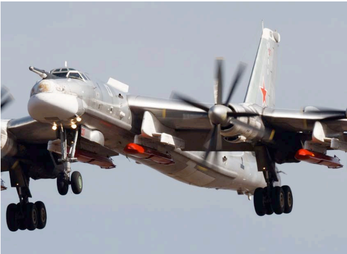
Russian Raduga Kh-101 low observable long range cruise missile during trials, carried by a Tu-95MS BEAR H. This stealthy cruise missile has been used repeatedly to attack targets in Syria (Anatoliy Burtsev).
