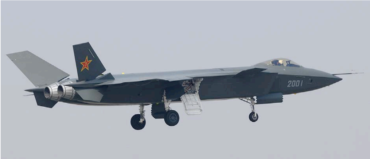
Prototype of the Chinese Chengdu J-20 supercruising high agility stealth fighter. The aircraft is now entering production, and was developed to compete with the US F-22A Raptor (PLA).
