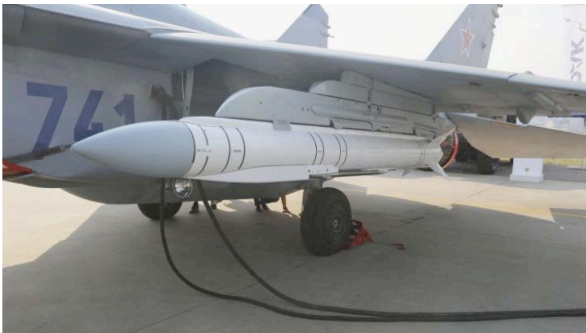
The Russian KTRV Grom E1/E2 glide-bombs are modelled on the US Small Diameter Bomb, but one variant has a motor to increase stand-off range (IHS Janes).
