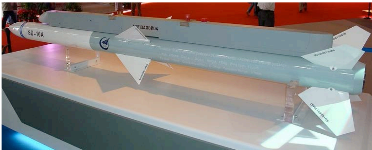
The Chinese LETRI SD-10/PL-12 “Sino-AMRAAM” is modelled on the US AIM-120 AMRAAM. Variants employ Russian Agat 9B-1348E active radar seekers, and a newer Agat dual mode seeker, providing also passive anti-radiation homing capabilities (Zhenguan Studio via APA).
