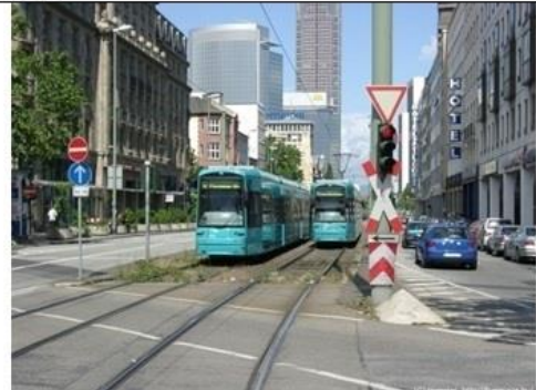
On dedicated track; car lanes gone
