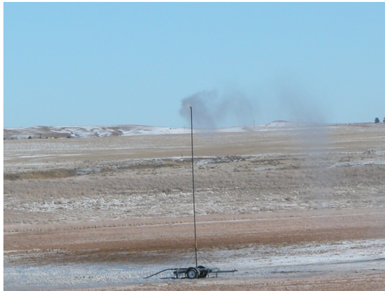
CBM produced water being aerated in the Powder River Basin, Wyoming
