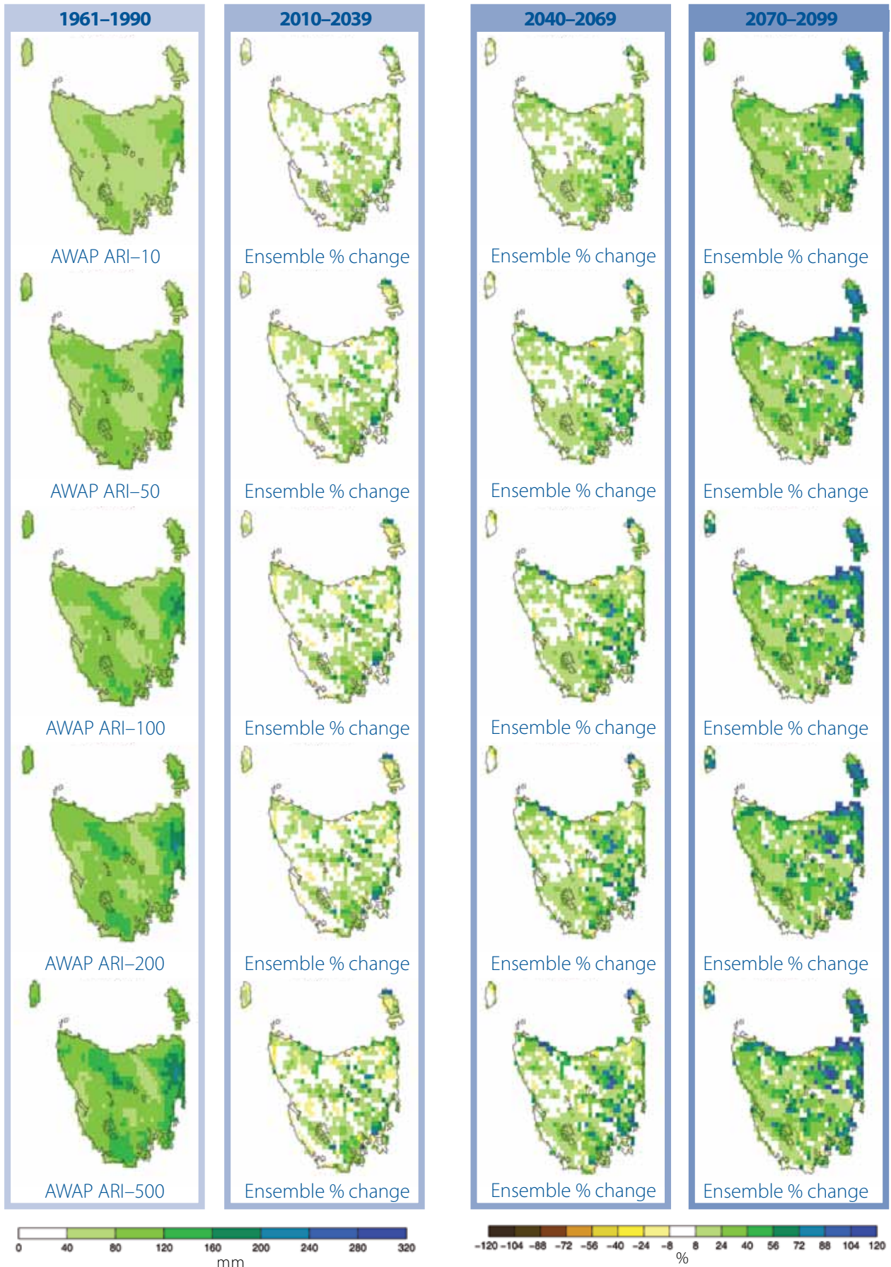
Figure 7.5 Magnitudes of 24-hour duration ARI-10 to ARI-500 (years) for 1961-1990 (left most panels) estimated from AWAP gridded observations (expressed in mm), with mean ARIs estimated from multi-GCM ensemble shown as the percentage change (right three panels) for 2010-2039, 2040-2069 and 2070-2099, relative to the AWAP 1961-1990 baseline using a generalized Pareto distribution. Multi-GCM ensemble ARIs estimated using the six downscaled-GCMs across Tasmania for the A2 emissions scenario.
