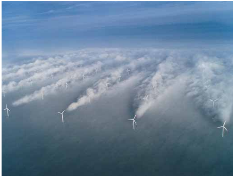
Figure 5: Downstream wake and turbulence effects
