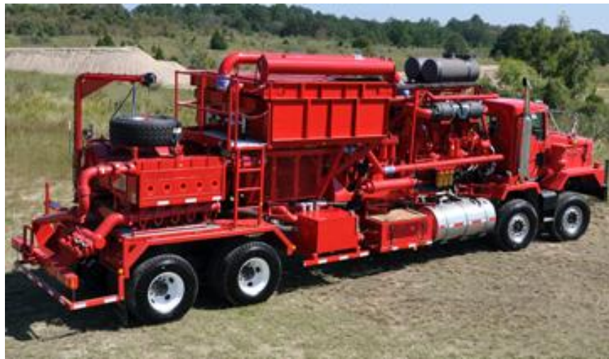
Photo 6.7 - Truck-mounted Hydraulic Fracturing Pump (New August 2011)
