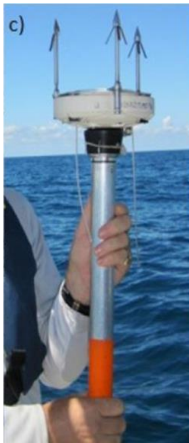
Fig. 8 Harpoon type tracking transmitter thrust into whales.
