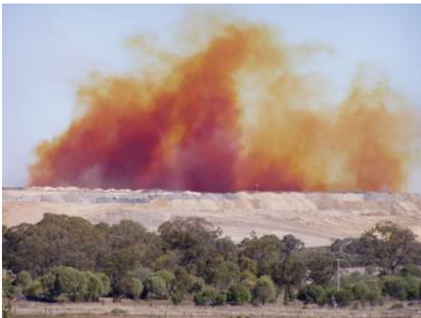
Fig 2 The view from a residence 1km from the Acland mine. Orange blast clouds- known to contain dangerous oxides of nitrogen are not uncommon. These can drift and settle in valleys distant from the mine.
