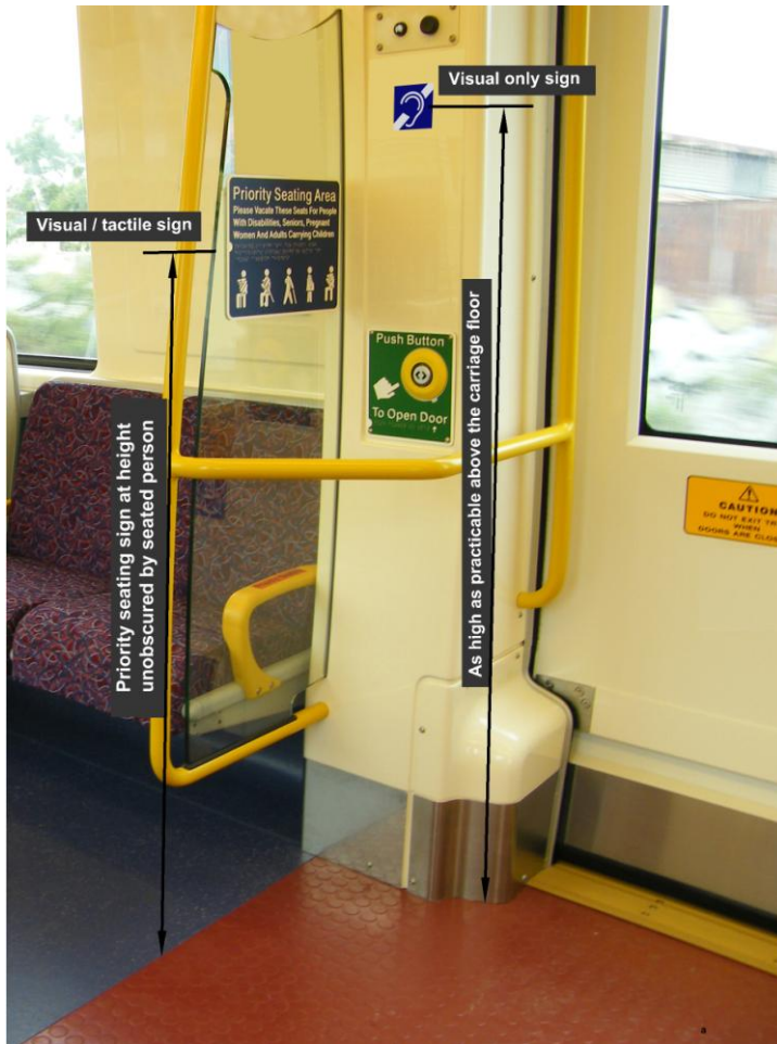
Figure 7.3.2. Examples of visual and visual / tactile sign location (dimensions in millimetres). Note: Sign text may be sentence or title case.
