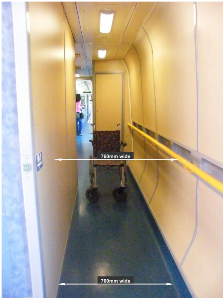
Figure 7.1.2. Example of 760 mm minimum clear width of access path where design constraints do not permit 850 mm minimum width. Note onboard carriage wheelchair used to provide direct assistance (dimensions in millimetres).
