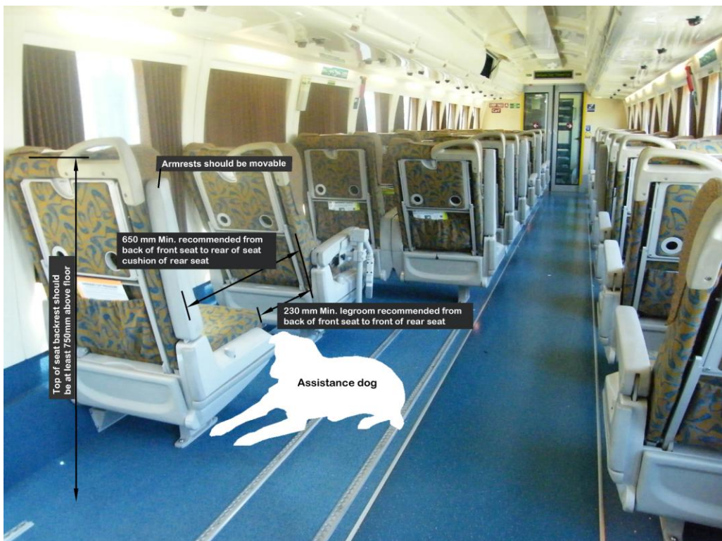
Figure 7.4.1.b. Examples of accessible seating dimensions and specifications (dimensions in millimetres).
