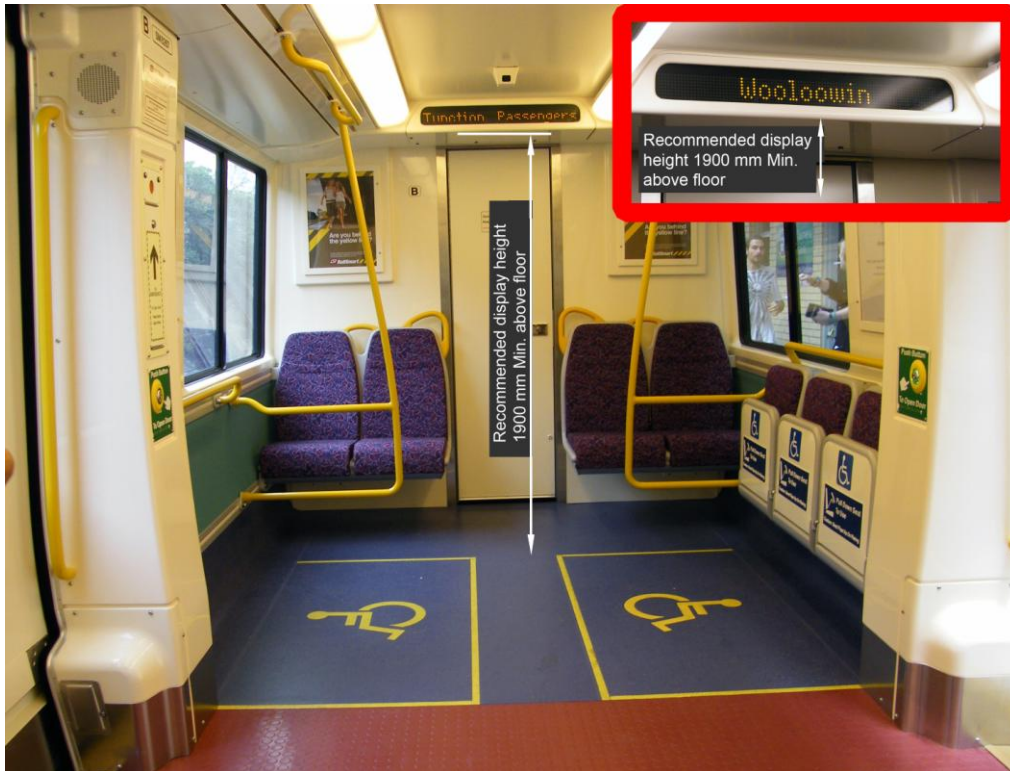
Figure 7.3.1. Examples of visual alternative destination display location and specifications (dimensions in millimetres).
