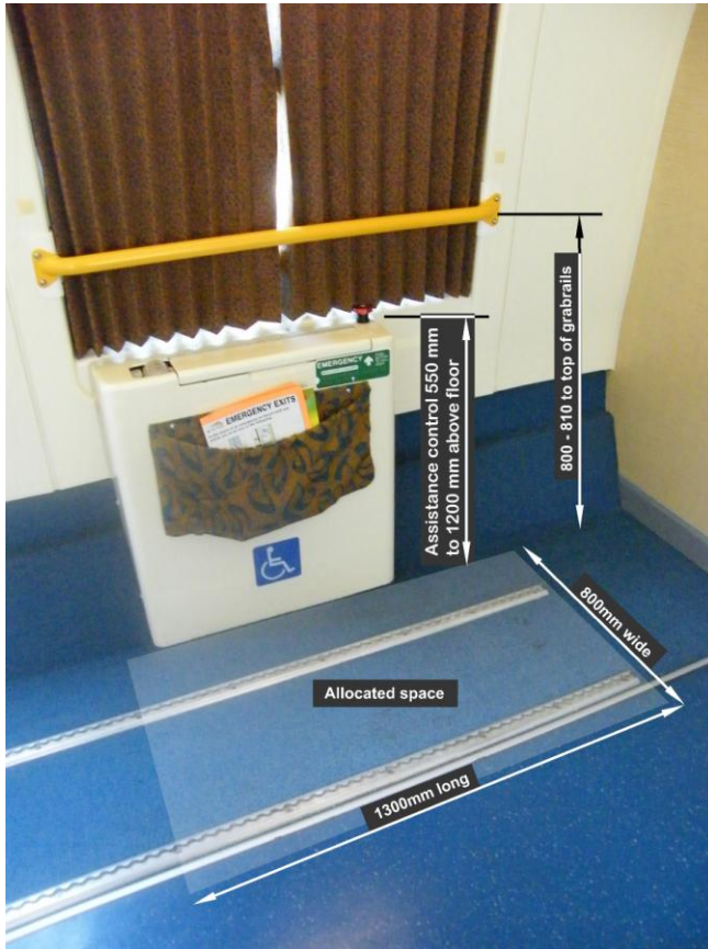
Figure 7.4.1.a. Examples of allocated space and call button dimensions and specifications (dimensions in millimetres).
