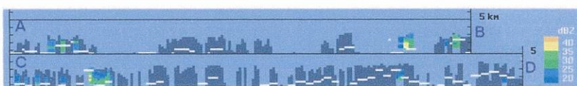
Fig. 5. Vertical cross section along the lines AB and CD in Fig. 2. The dark gray areas represent clouds. The vertical extent of the clouds is converted from the VIRS-measured cloud-top temperatures. The colors represent the precipitation reflectivity in dBZ as measured by the TRMM radar. The white line is the brightness temperature of the TMI 85-GHz vertical polarization ( T_{85} ), plotted at the altitude of that temperature. A lower T_{85} value is represented as greater height of the white line, and in nonprecipitating clouds it means greater cloud water content. The T_{85} and actual cloud-top temperature have different physical meanings.
