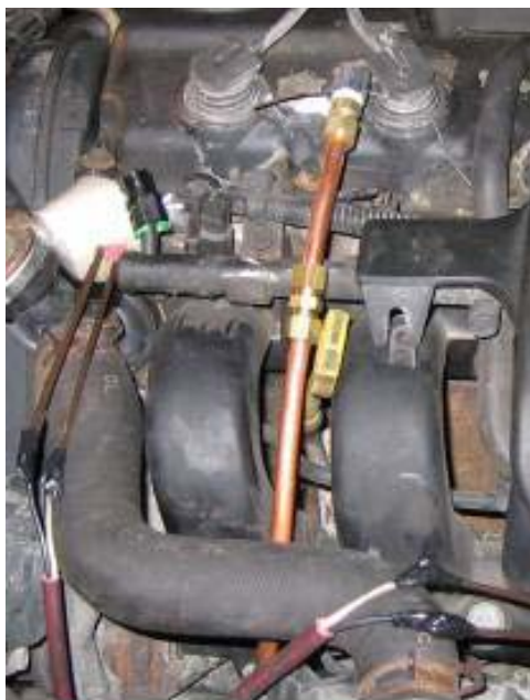
Figure 4-15: Automobile engine compartment fire initiation device.
