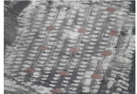
Sonoma Coal Mine on Coral Creek Beside Bowen Developmental Rd. Shot firing/Blasting preparation.
