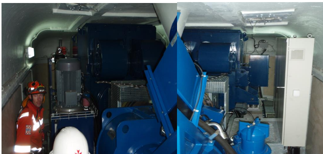
Figure 6 & 7- The inside of the Nacelle depicting the amount of space taken up by the gearbox and generator
