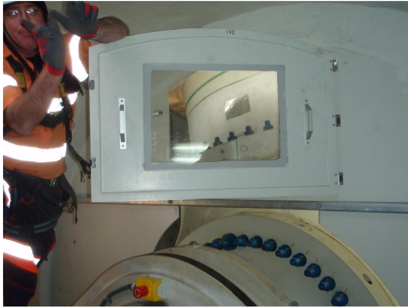
Figure 8- Access door from the Nacelle to the Hub. Note shaft connection underneath access door
