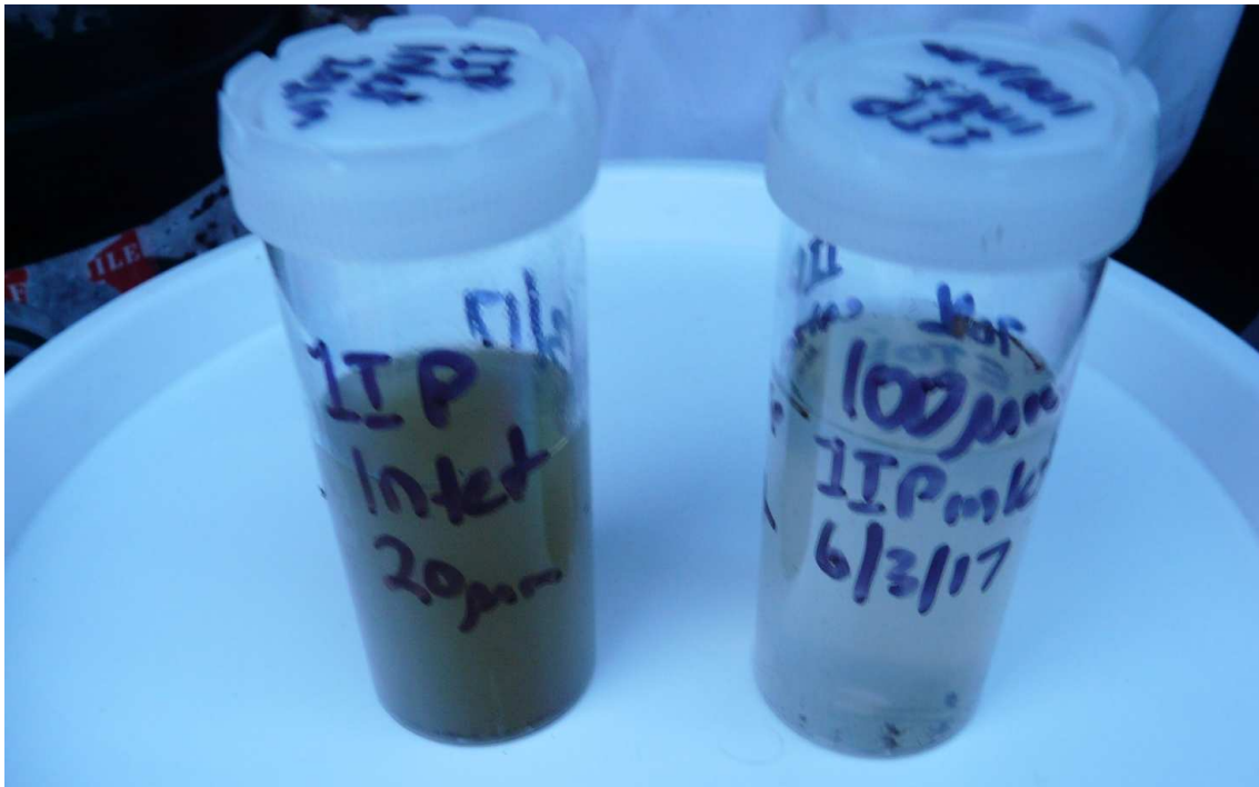
Figure 11. Comparison between samples collected from the junction between the IIP inlet and the Logan River in a 15-20 \mu\text{m} plankton net (left) and a 100 \mu\text{m} plankton net (right). Much more phytoplankton and particulate matter was sampled using the 15-20 \mu\text{m} net, suggesting it may be a useful method of sampling environmental/particle associated WSSV.
