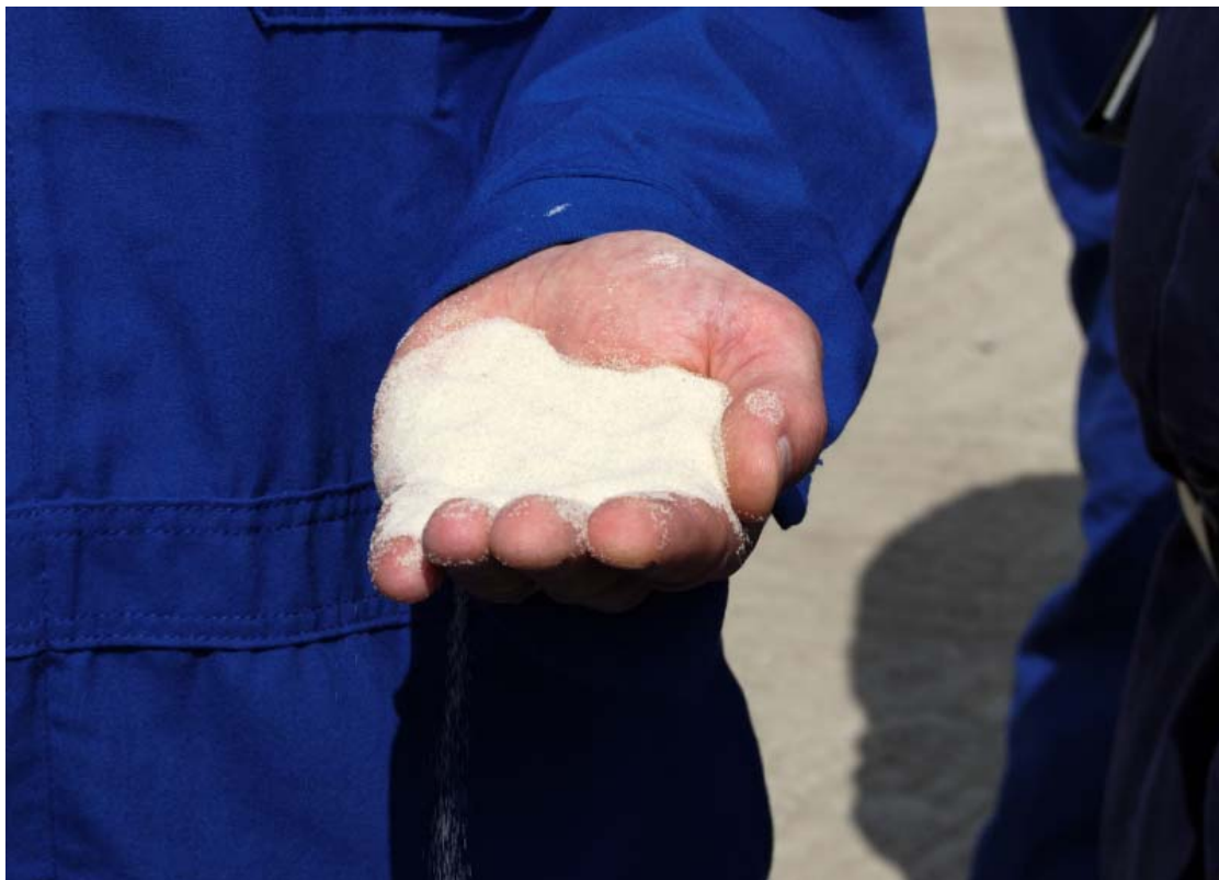
Photo 5.17 - Sand used as proppant in hydraulic fracturing operation in Bradford County, PA
