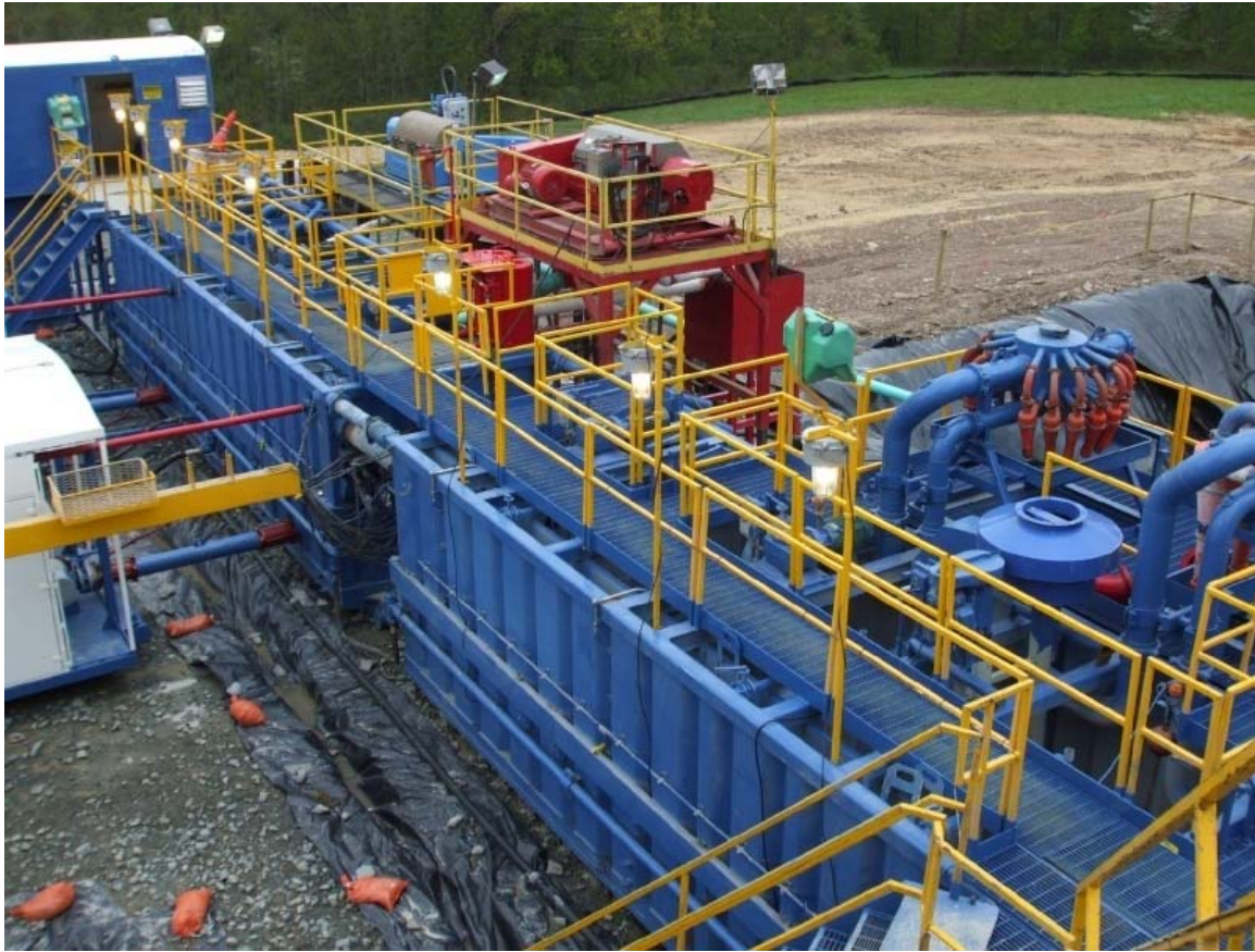
Photo 5.16 - Drilling rig mud system (blue tanks)
