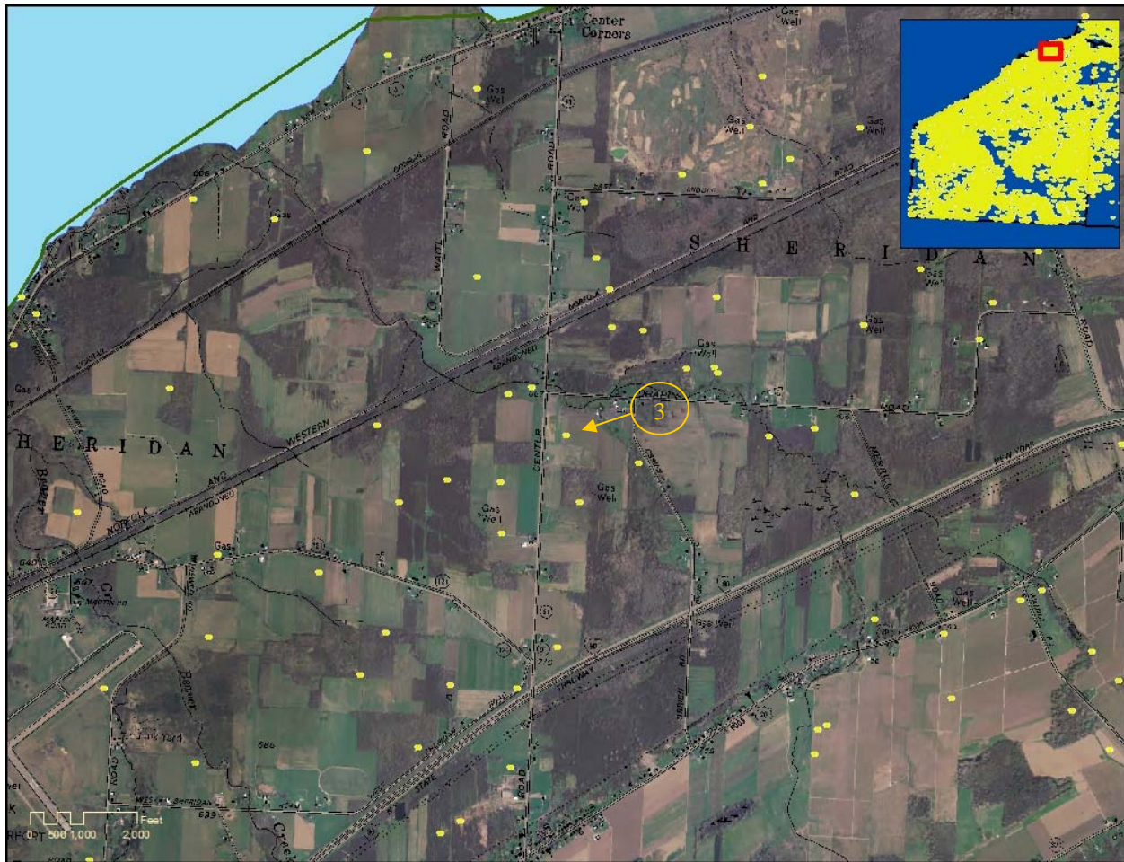
Photo 5.11 a & b The map above shows 77 wells. Well #3 (API Hole number 16427) identified in the map above, and shown in the photo below, was completed in the Town of Sheridan, Chautauqua County in 1981 and was drilled to a depth of 2,012 feet. The map indicates that the nearest producing well to Well #3 is 1/4 mile away.
