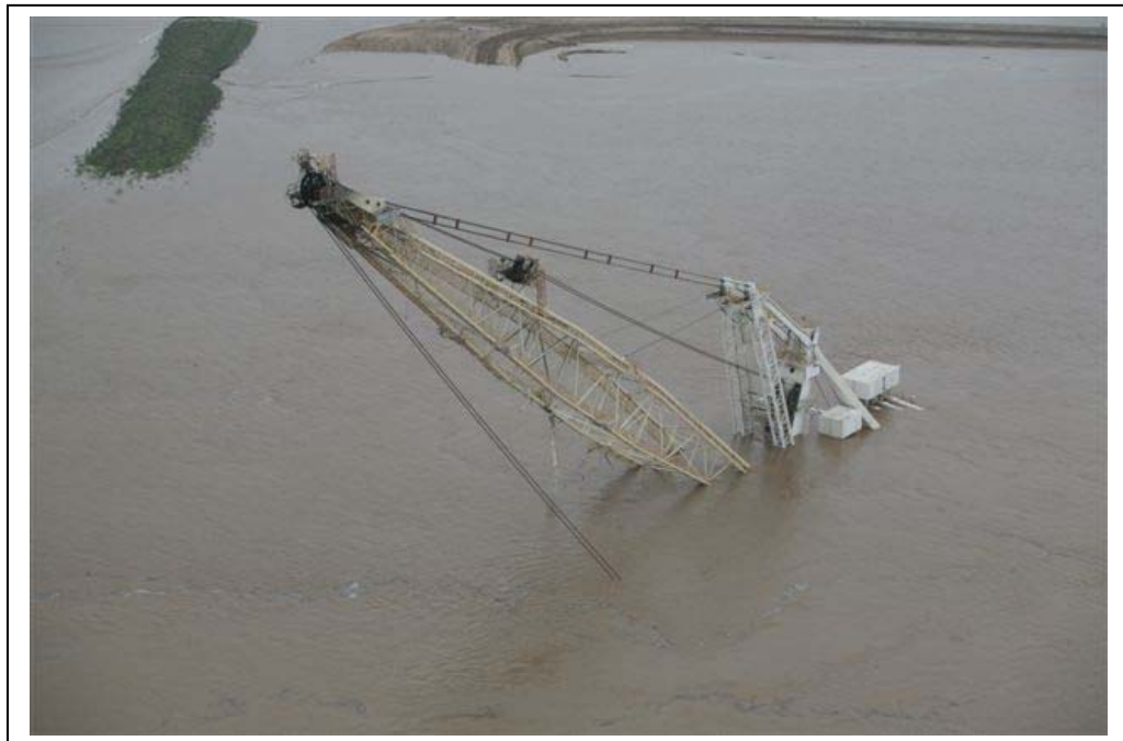
10 story dragline submerged at Ensham. Remains of levee bank top left.
