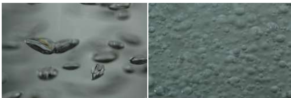
Figure 6. Nitrogen bubbles formed in a water column at a frit: in pure water (left photo) and in salt solution at 0.2M NaCl (right photo), for the same flow rate.
