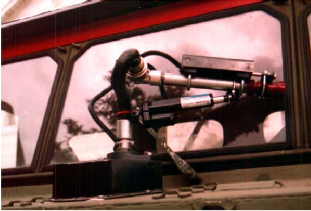
Figure 2 - Remote controlled monitor - Roscommon Equipment Center project No. 58
