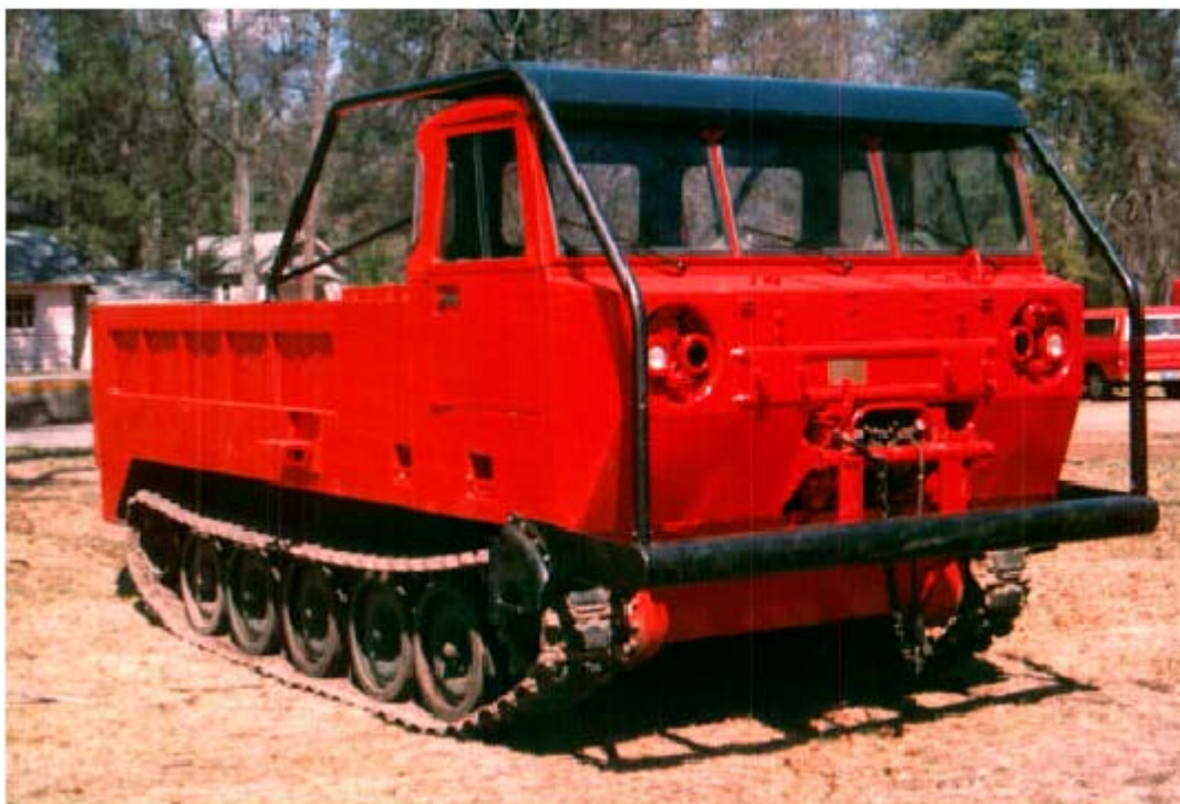
Figure 1 - M548/M1015 full tracked fire fighting vehicle developed at Roscommon Equipment Center.
