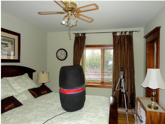
Figure 3: Microphone in windscreen monitoring room center in study home.
