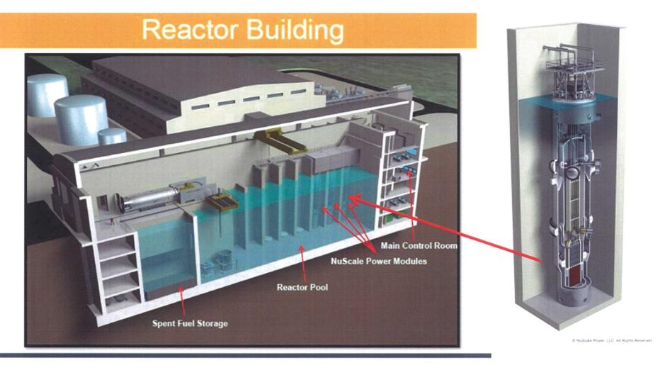
Up to twelve x 50MWe modules. Natural circulation, reactor underground Passive safety systems – cooled indefinitely without attention – "indefinite coping time"
