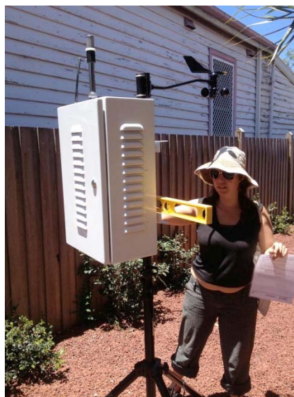
Picture 1: Representative testing Oris dust monitor
